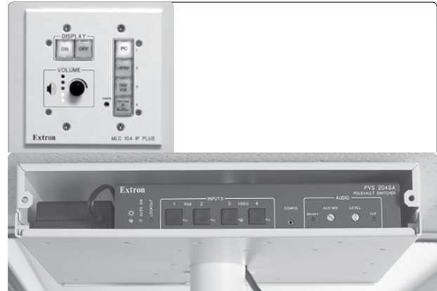
2a) Turn on the MLC 104 IP Plus controller and the PVS 204Sa switcher
